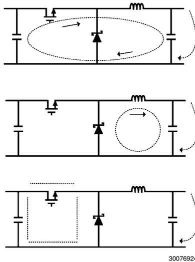
FIGURE 3. Current Flow in a Buck Application
